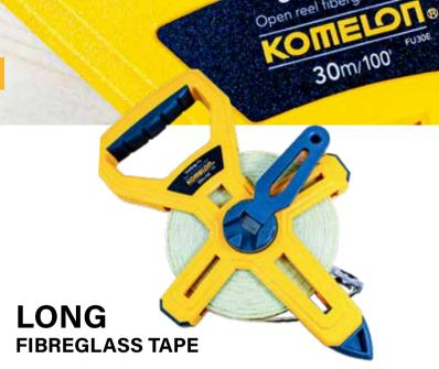
Komelon Long Fibreglass tapes come in 30m/100ft, 50m/165ft, 100m/330ft lengths. The ABS open frame has a gear driven winding handle and 2 steel rollers to allow the blade to return without twisting. The blade is made of 16,000 strand fibreglass to prevent stretch and it's the only fibreglass tape on the market to have Class 2 accuracy.
