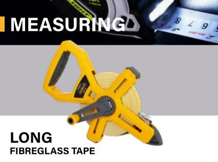
Komelon Long Fibreglass tapes come in 30m/100ft, 50m/165ft, 100m/330ft lengths. The ABS open frame has a gear driven winding handle and 2 steel rollers to allow the blade to return without twisting. The blade is made of 16,000 strand fibreglass to prevent stretch and it's the only fibreglass tape on the market to have Class 2 accuracy.
