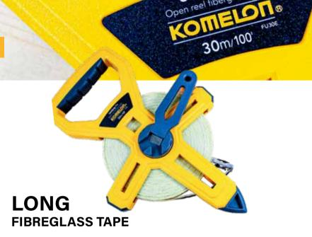
Komelon Long Fibreglass tapes come in 30m/100ft, 50m/165ft, 100m/330ft lengths. The ABS open frame has a gear driven winding handle and 2 steel rollers to allow the blade to return without twisting. The blade is made of 16,000 strand fibreglass to prevent stretch and it's the only fibreglass tape on the market to have Class 2 accuracy.
