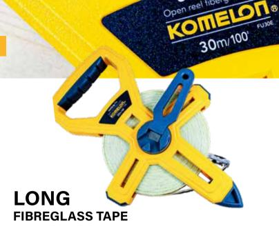
Komelon Long Fibreglass tapes come in 30m/100ft, 50m/165ft, 100m/330ft lengths. The ABS open frame has a gear driven winding handle and 2 steel rollers to allow the blade to return without twisting. The blade is made of 16,000 strand fibreglass to prevent stretch and it's the only fibreglass tape on the market to have Class 2 accuracy.
